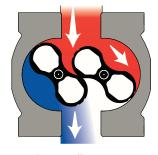
As the impellers continue to turn, the volume of gas in the left cavity is discharged. Simultaneously, gas is entering the space between the right impeller and housing.
